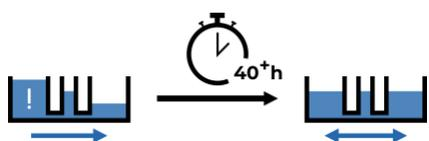
When adjacent chambers are loaded with different volumes of fluid for the purposes of driving a unidirectional flow across the adjoining microchannels, we refer to this as “**asymmetrical volume loading**” of the chambers. The unidirectional flow
