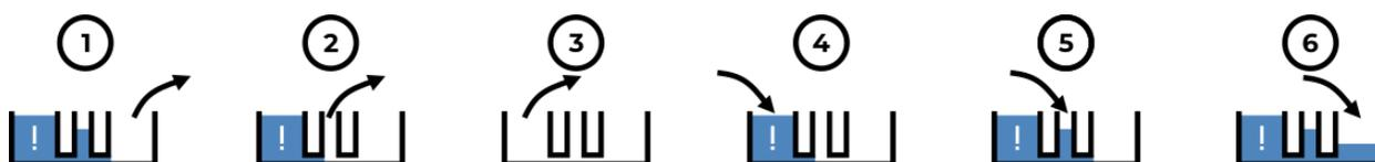
In addition to chamber isolation purposes, asymmetrical volume loading of chambers is useful when it is desirable to induce a flow through the microchannels. For example, this might be the case, when coating the microchannel surfaces or chemically fixing neuronal projections located within the microchannels. Also, asymmetrical volume loading is necessary to allow antibody access to epitopes located within the microchannels when performing immunohistochemical staining procedures.
